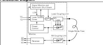
The receiver component converts the optical serial data into PECL compatible electrical data (RD and RDnot). The Signal Detect (SD, active high) shows whether optical data is present<sup>(1)</sup>.
